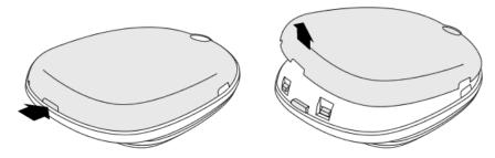
**3** To remove the battery, lift the battery using the battery lift tab.
